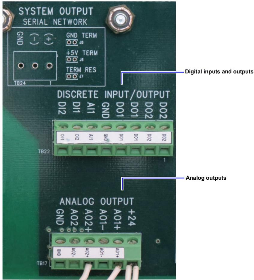
Figure 3-4. System Input and Output Communications
