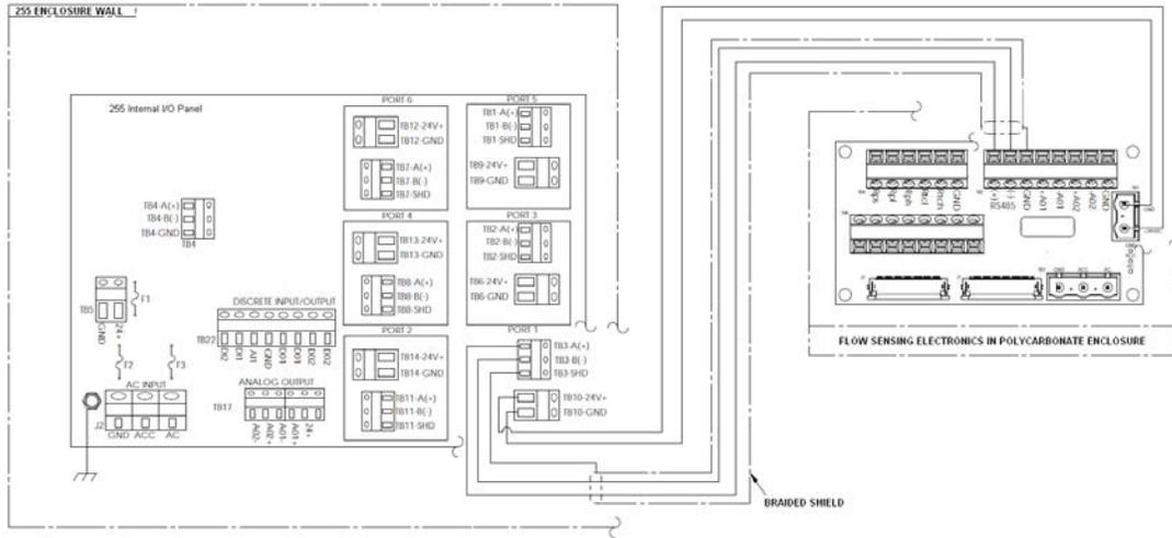
Figure 2-14. Example — Wiring from a Series 255 to a Single-Point 454FTB (Transmitter-Separate, polycarbonate)
