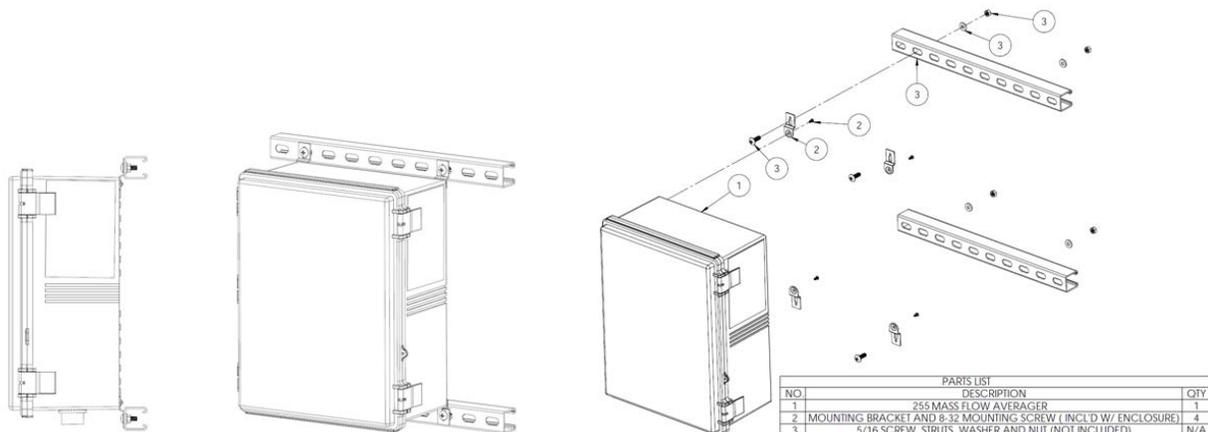
Figure 2-1. Polycarbonate Enclosure — Rail-Mounted Example
