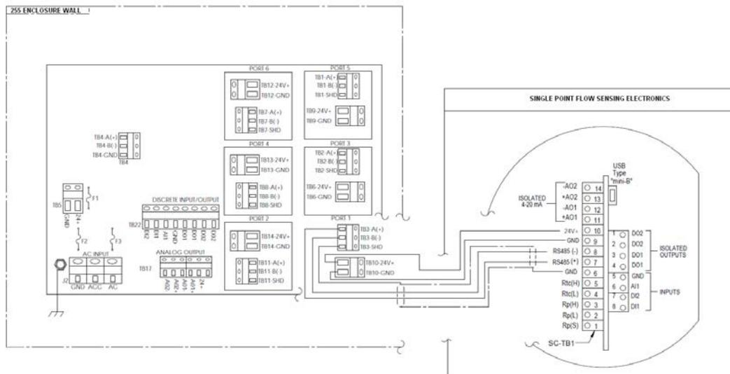
**Figure 2-13. Example — Wiring from a Series 255 to a Single-Point 454FTB (Transmitter-Attached)**
