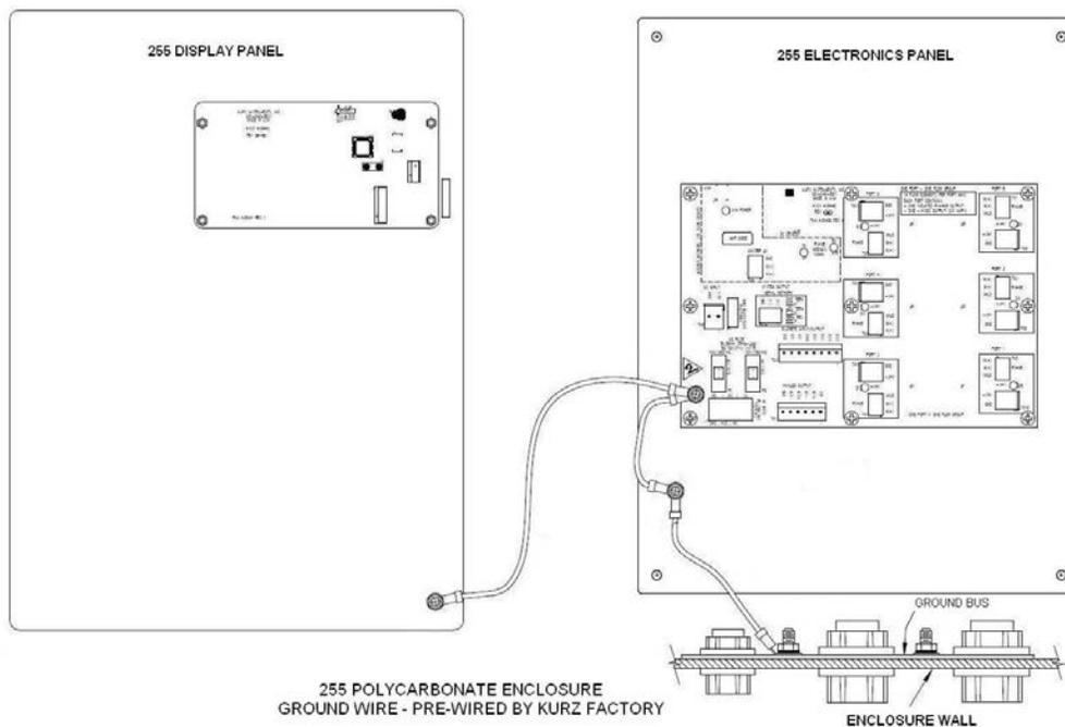
**Figure 2-8. Ground Bonding for Polycarbonate Enclosures**
