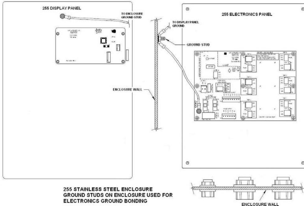
**Figure 2-9. Ground Bonding for Stainless Steel Enclosures**
