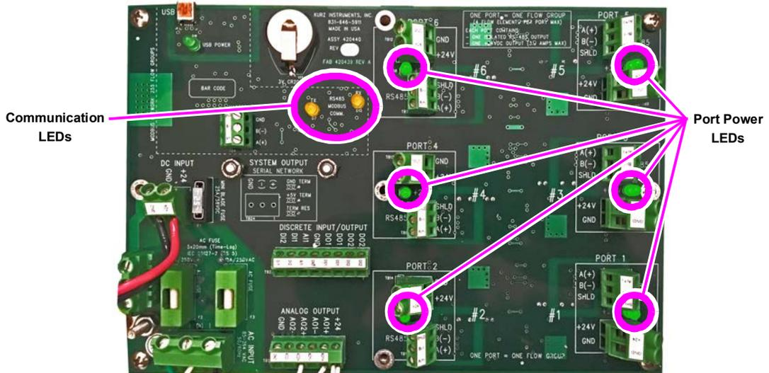
Figure 2-20. System Board LEDs
