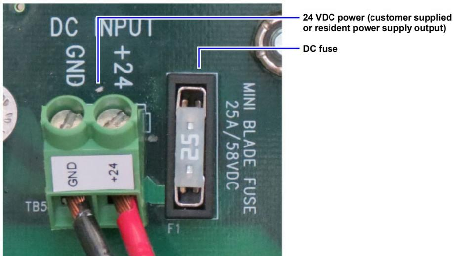
Figure 3-3. DC Power Connections
