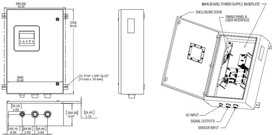
Figure 2-4. Stainless Steel Enclosure for Hazardous Locations
