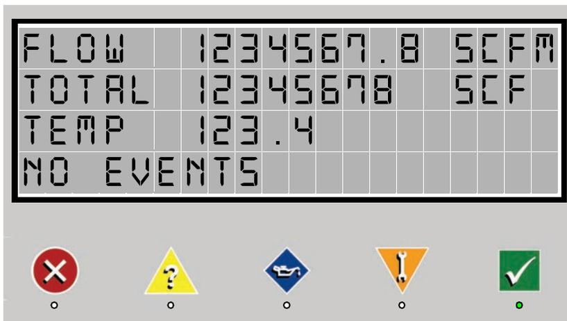
Figure 2-21. Example — Front Panel Status Indicators, System Operating Without Error
