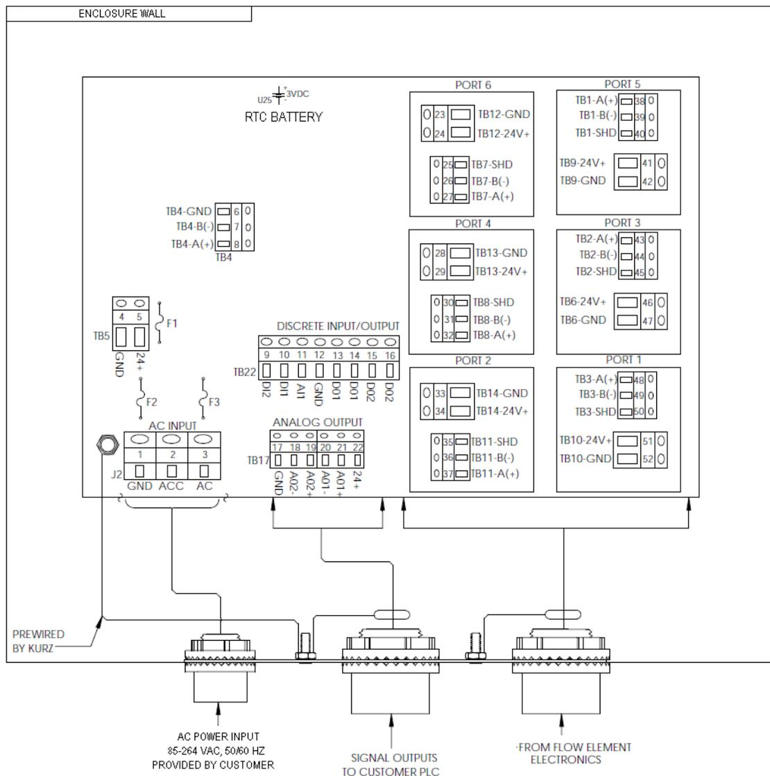
Figure 2-10. Terminal Connection Layout
