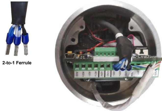
**Figure 2-17.** Example of 2-to-1 Ferrule used with a Single-Point Flow Meter
