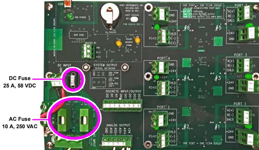
Figure 2-22. Location of System Board Fuses
