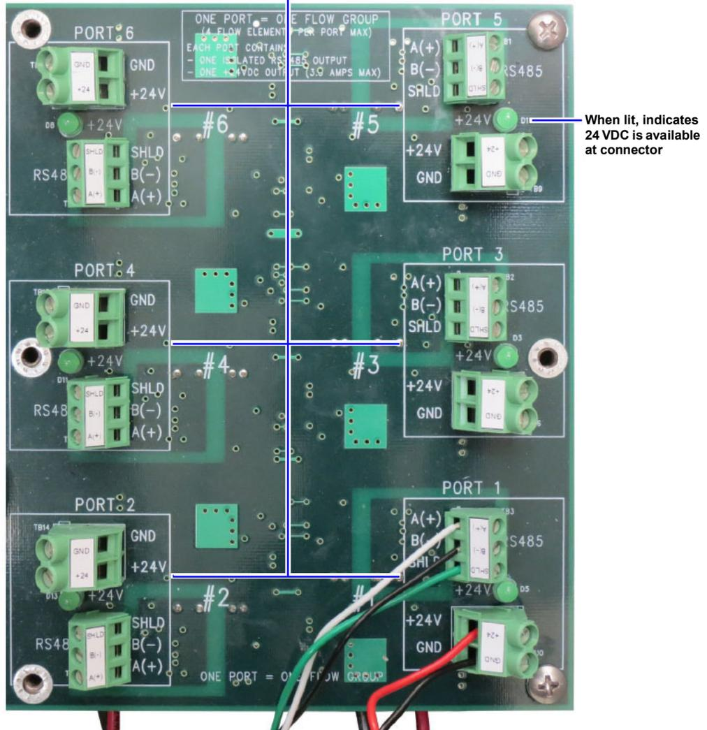
Figure 3-6. Sensor Power and Communications Connections
