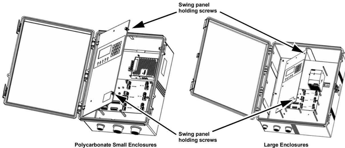
**Figure 2-11. Swing Panel Holding Screws**
