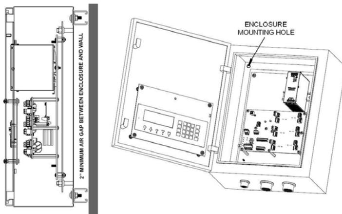
**Figure 2-2. Stainless Steel Enclosure — Inside Mount Example**
