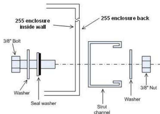
**Figure 2-3. Stainless Steel Enclosure — Mounting Hardware Stack Detail**
