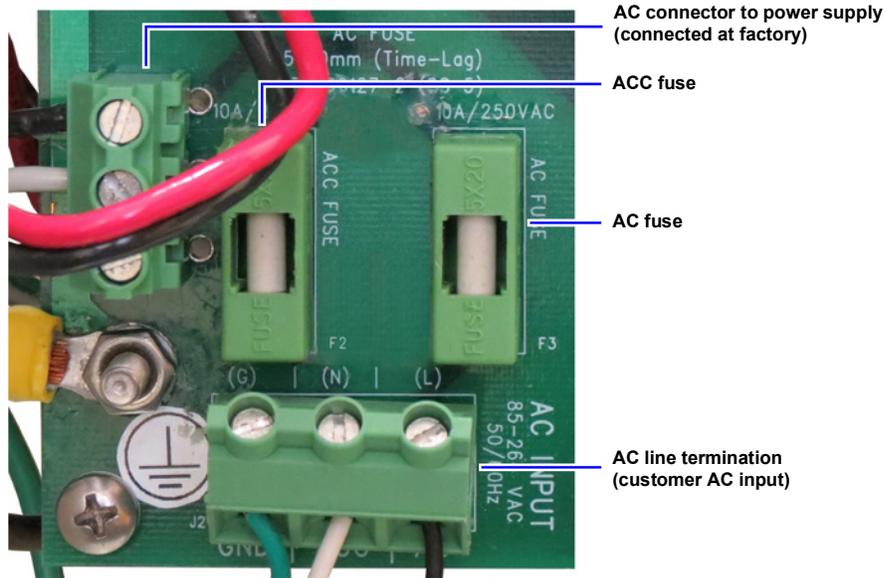
Figure 3-2. AC Power Connections
