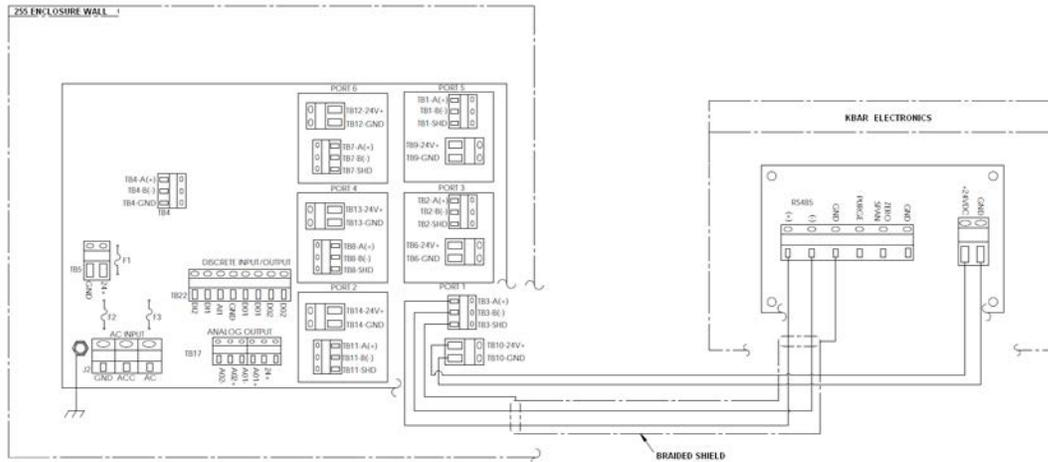
**Figure 2-12. Example — Wiring from a Series 255 to a Multipoint K-BAR 2000B**
