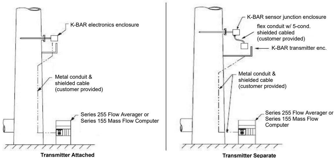
**Figure 2-14. K-BAR 2000B electronics configuration examples**
