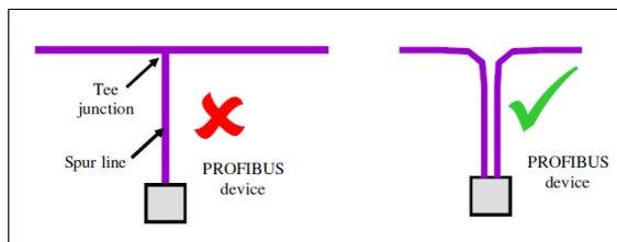
Repeaters can be used to avoid spur lines, by isolating the branch cable that goes to a device. This is especially true for devices that have non-standard bus connectors.
