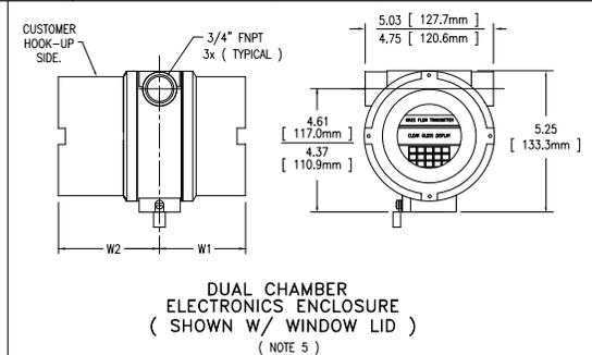
TABLE 1 SERIES 504FTB IN-LINE MASS FLOW TRANSMITTERS DIMENSIONS
