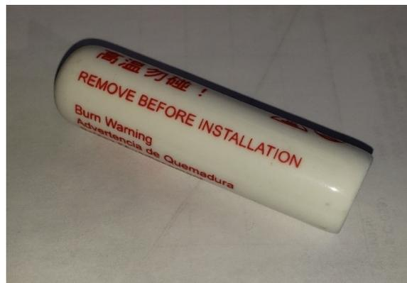
Figure C-2. Example sensor window cap for Zero Flow Air test
