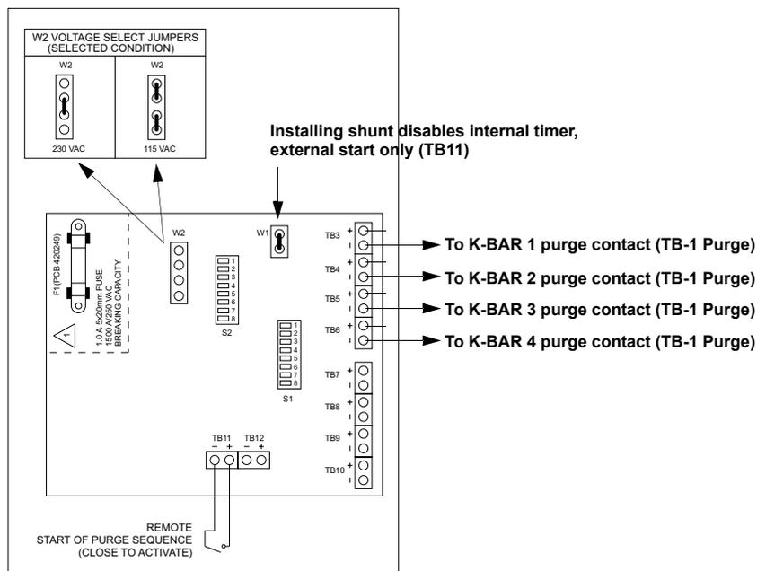
**Figure 2-21. K-BAR 2000BP multipoint controller circuit board example**
