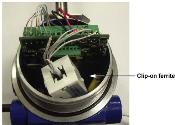
**Figure 2-22. Clip-on ferrite for I/O wires**
