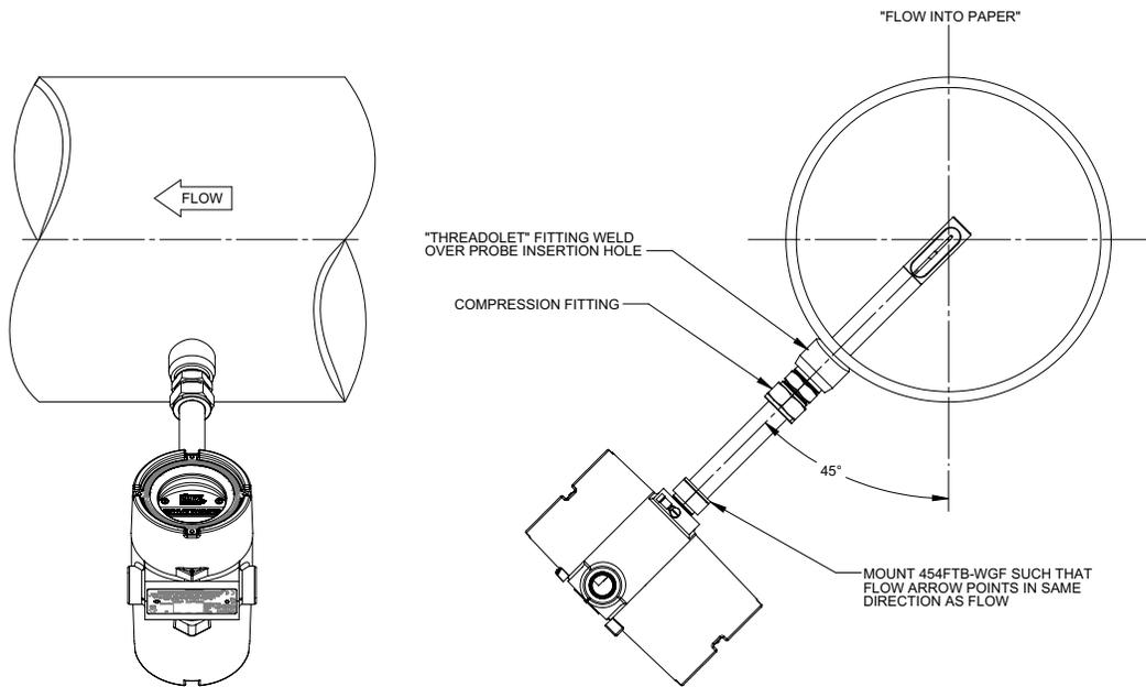
**Figure 2-3. Mounting and sensor criteria for the 454FTB-WGF**
