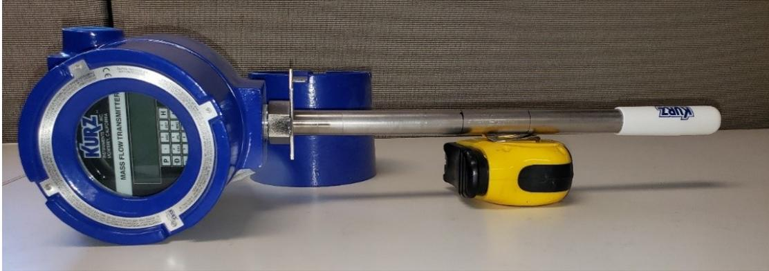
Figure C-4. Probe with flow arrow up, level, window cover in place
