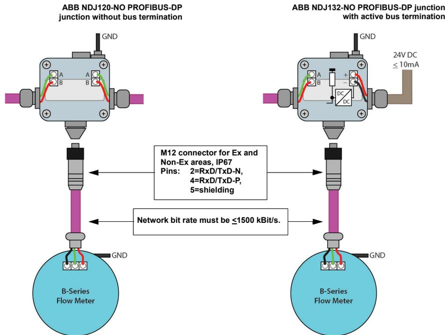
**Figure 4-4. Recommended Wiring Connection with a Spur Line**
