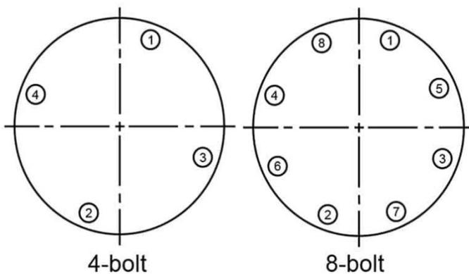
**Figure 2-13. Bolt tightening sequence for 4-bolt & 8-bolt flange**
