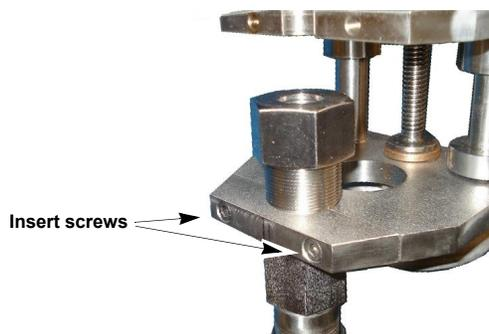
**Figure D-4. Lower guide block**
