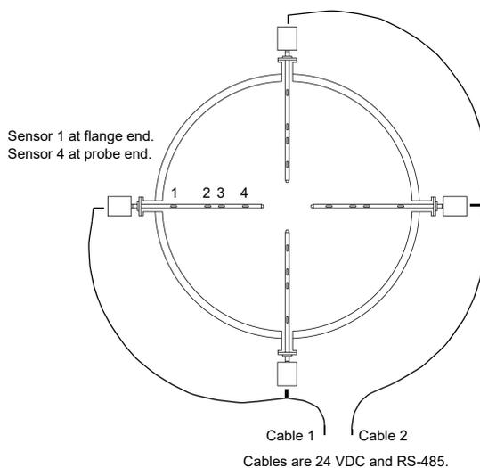
**Figure 2-23. K-BAR example using Modbus communication**
